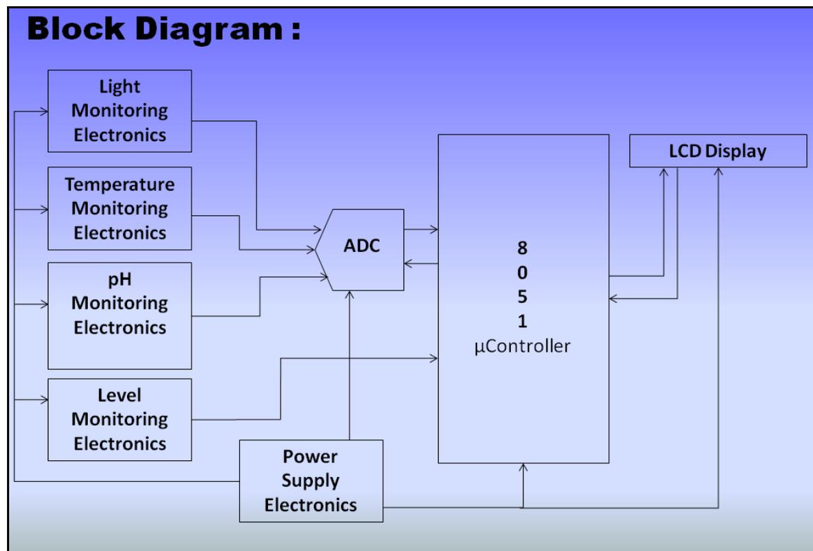
Fig. 1: Block Diagram of Liquid Chamber Monitoring System
