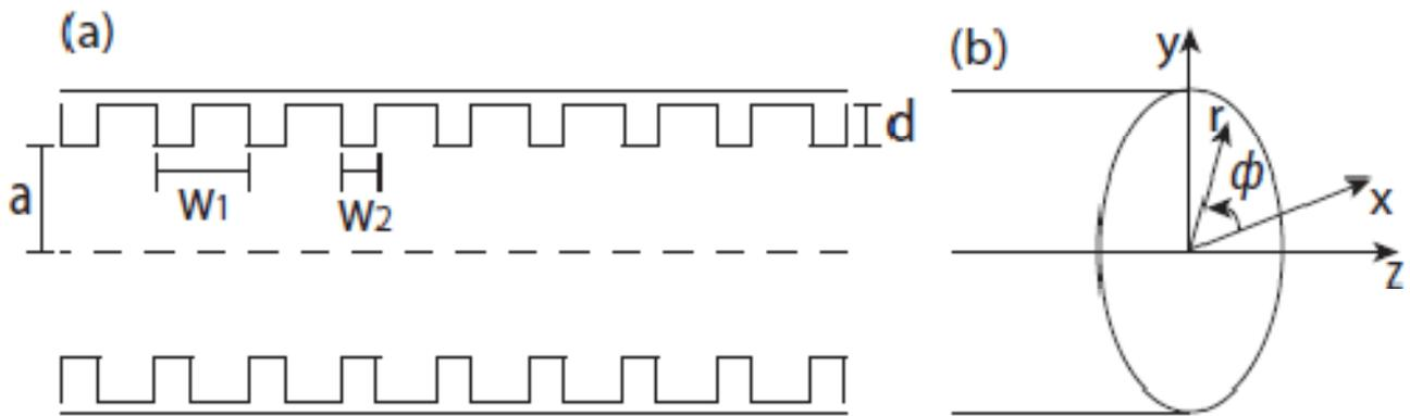
Fig.1 (a) A cylindrical corrugated waveguide with a radius of a. The corrugations are defined by w1, w2, and d. For low loss characteristics the corrugation depth is  $d = \lambda/4$ . (b) An illustration of the variables in the cylindrical geometry.
