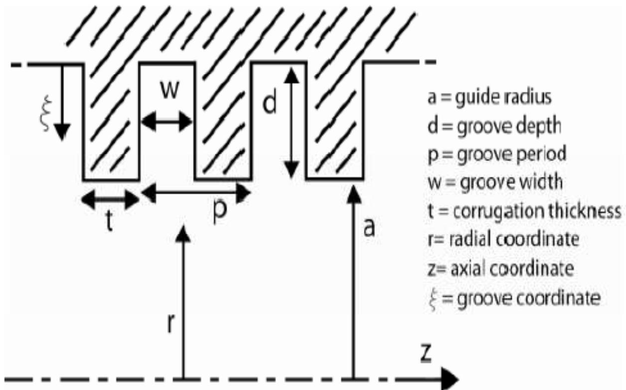
Fig -2: Illustration of circular corrugated waveguide [1]
