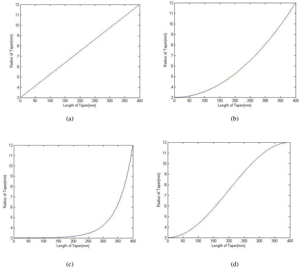
Fig.1 Shape profile of circular waveguide tapers
