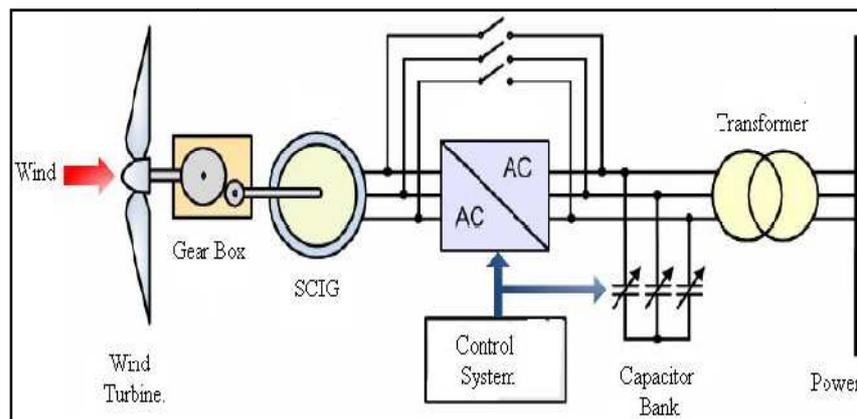
Fig.7 fixed speed wt connected directly to power grid with SCIG
