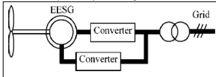
Fig.11 Electrically excited synchronous generator
