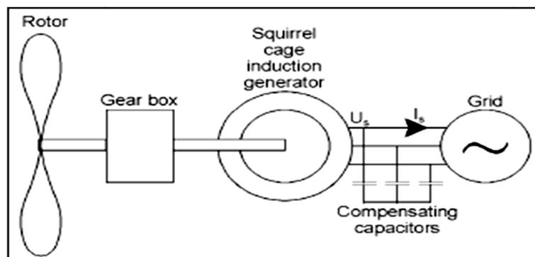
Fig.4 squirrel cage induction generator
