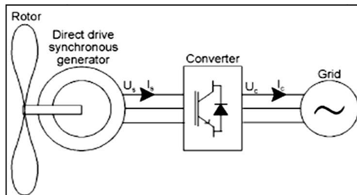
Fig 6:Direct drive synchronous generator
