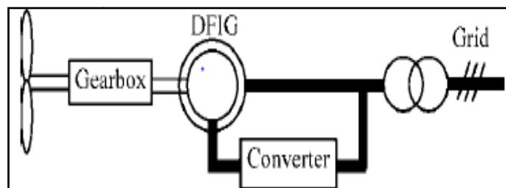
Fig.10 Variable speed concept with a partial-scale power converter
