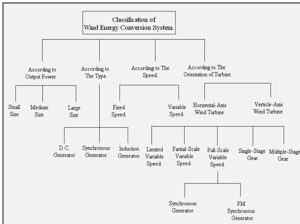
Fig. 2 classification of wind energy conversion system
