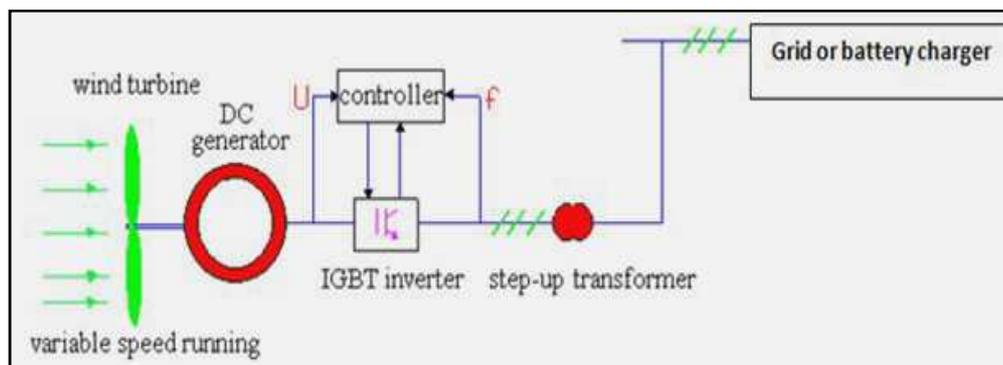
Fig. 3 dc generator wind turbine
