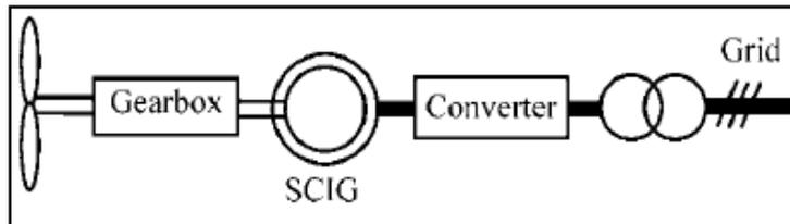
Fig.13 Variable speed multiple-stage geared concept with a full-scale power converter
