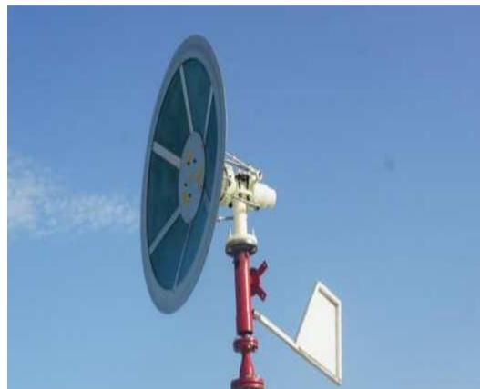
Fig.17 Bladeless wind turbine
