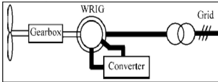
Fig.8 variable speed WT connected directly to power grid with DFIG
