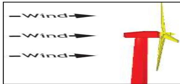
Fig. 15 Down wind turbines
