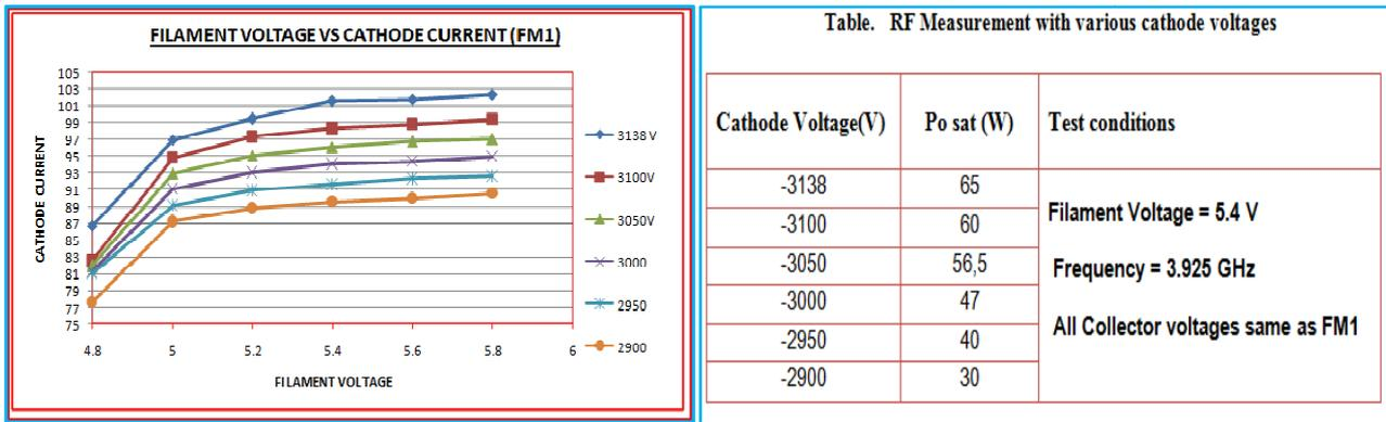
FIG.2 Experiment results of Cathode voltage reduction
