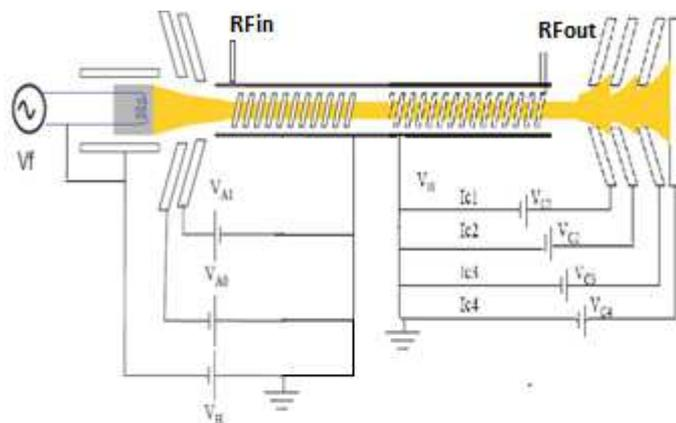
Fig. TWTA, EPC-TWT interface diagram
