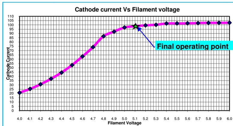
Fig.3 Final filament operating point recommended
