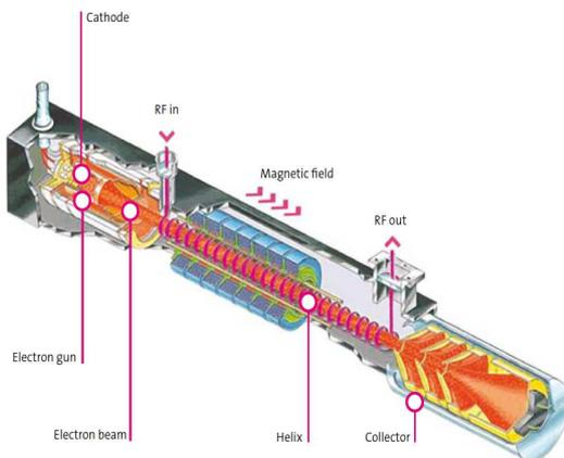
Fig. Cross section of TWT
